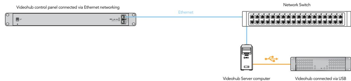
**Connection method 2.** Connecting to a USB-attached Videohub via a network switch.
