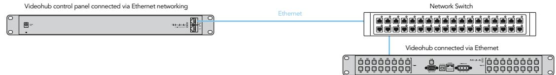
**Connection method 1.** Connecting to an Ethernet-equipped Videohub via a network switch.
