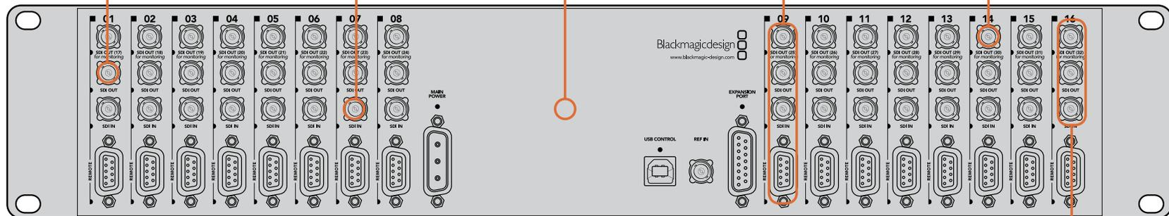
RS-422 control ports switch between in for edit systems, or Out for decks
