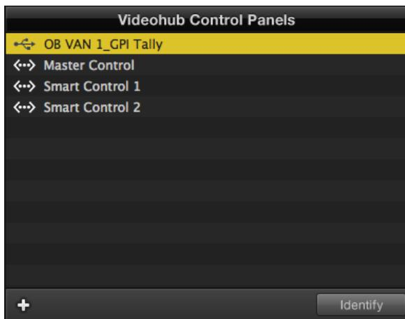
GPI and Tally Interface connected via USB
