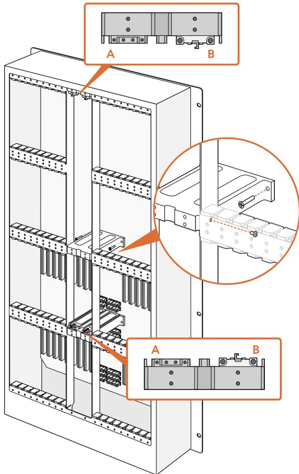
**Step 5:** Stand the supporting bridge so the holes in its left and right feet are positioned over the corresponding mounting holes on the motherboard standoffs. The card guides should face the lower supporting bridge at the bottom of the crosspoint slots.
